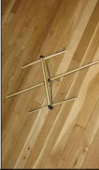
6. Place two more vertical sticks at each side of the bottom horizontal stick at its center. Insert the band into the slot of each stick and firmly secure them with a cap.
